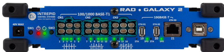
H-MTD Connectors for High-speed 1000BASE-T1 networks
