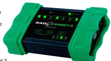
When configured as a media converter, the RAD Comet 3 can bridge between any of its 3 Ethernet physical layers. This is useful for connecting a PC to an Automotive Ethernet device for observing network activity in Wireshark or Vehicle Spy. It is also useful for integrating a 10BASE-T1S device or network into a 100/1000BASE-T1.
