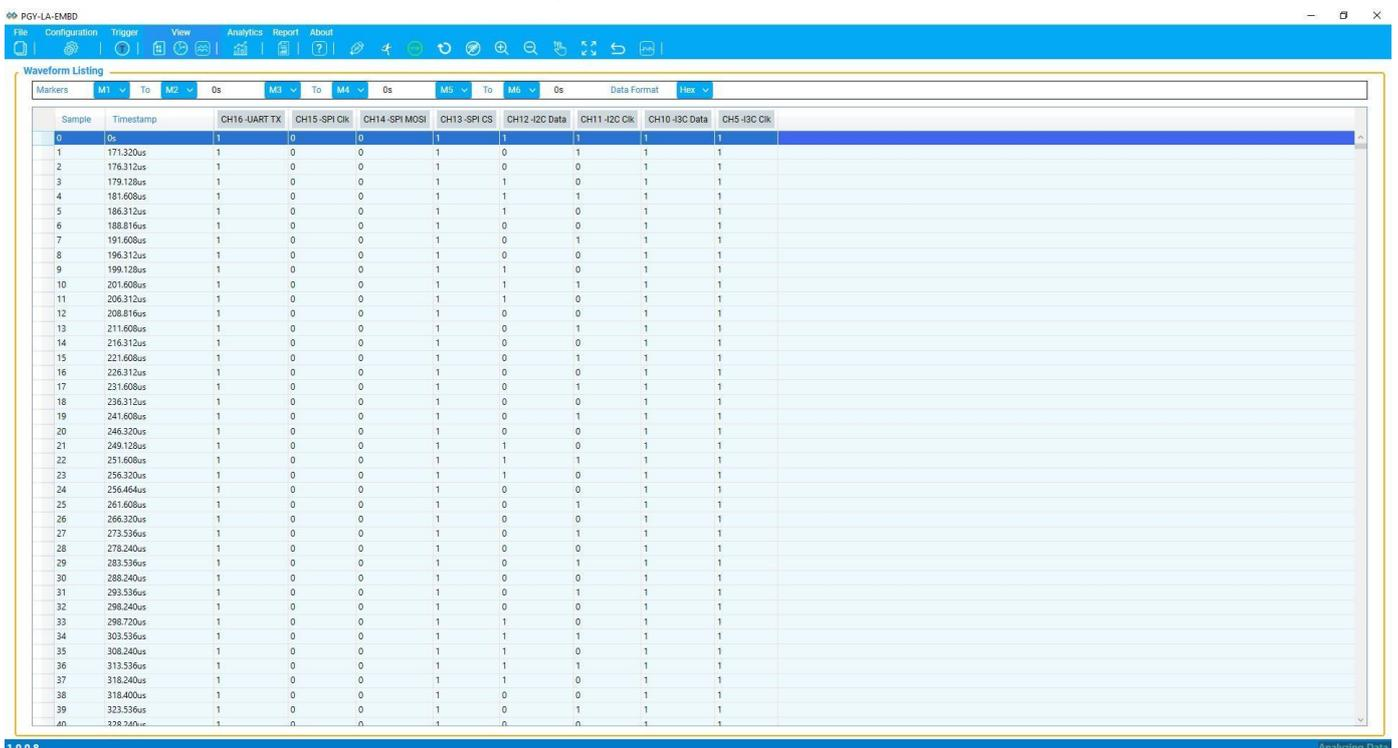
The screenshot displays a Waveform Listing interface. The top menu includes File, Configuration, Trigger, View, Analytics, Report, and About. The main table shows a list of captured data points with columns for Sample, Timestamp, and various channel data (CH16-UART TX, CH15-SPI Clk, CH14-SPI MOSI, CH13-SPI CS, CH12-I2C Data, CH11-I2C Clk, CH10-I3C Data, CH5-I3C Clk).
