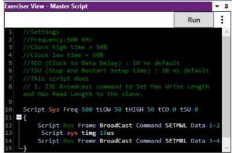
PGY-I3C-EX-PD supports I3C traffic generation using GUI and Script. Users can perform simple traffic generation using the GUI to test the DUT. Script-based GUI provides flexibility to emulate the complete expected traffic in the real-world including error injections. In the below sample script users can generate I3C traffic as below:
