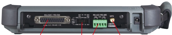
RS-232C/RS-530 measurement port TTL measurement port / external trigger terminal RS-422/485 measurement port GPS antenna connector
