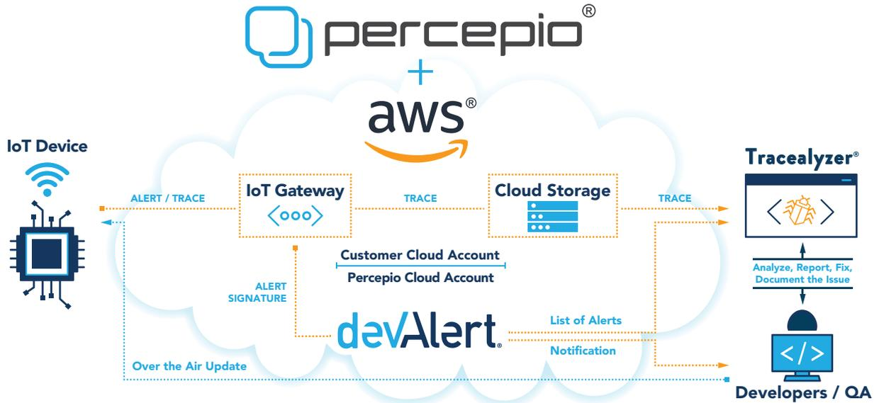
When triggered, the DevAlert agent on the device uploads a small report to the developer's AWS account. The solution protects the data transmission by using the AWS IoT infrastructure and messaging, which employs best practices for authentication and encryption, such as X.509 certificates and TLS.
