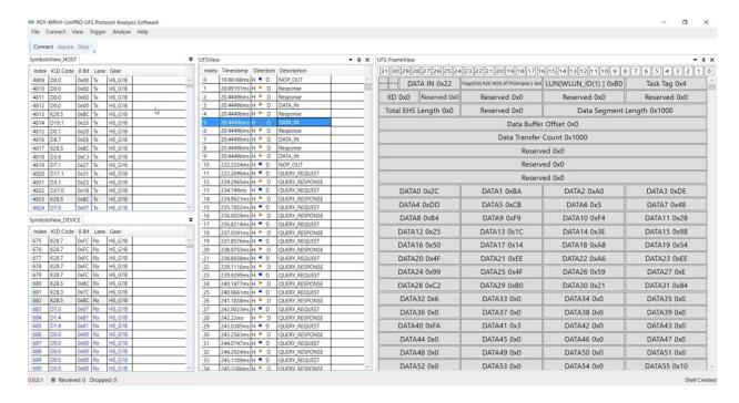
UFS layer view has UFS view and UFS Frame view. UFS view list all the UFS packets and UFS Frame view provides selected packets decoding at UFS packet format.
