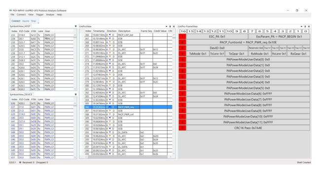
PGY-UFS3.0-PA UFS Protocol Analysis offers multilayer of protocol view with flexibility to link all views for easy correlation of data. Selected packets details are displayed in a format which is similar to specification document format for easy correlation. This view provides bit level information to analyze the communication between UFS host and UFS memory.
