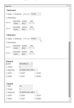
PGY-UFS3.0-PA UFS Protocol Analyzer offers powerful hardware-based trigger capabilities allowing design and test engineer to capture the protocol activity at specific event. Hardware based algorithm computes the CRC values in real time and can trigger on CRC error. Triggering on any of the UniPro layer protocol packet or Bad alignments (Improper marker values) reduces the debug time
