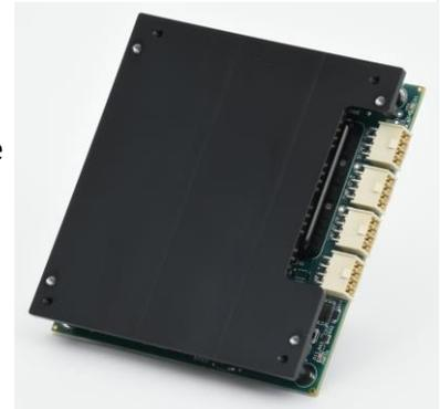
Integrated heat spreader supplied with all models
