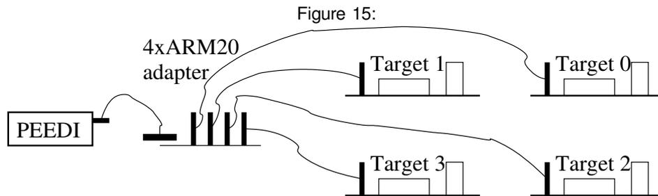
The multiple core (extra license is required) support allows you to debug/program up to 4 independent targets using only single PEEDI. The targets must be chained using the multiple core cable adapter available from Ronetix:
