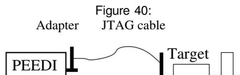
All adapters are mounted on the PEEDI JTAG connector and next the target cable is connected to the given adapter:
