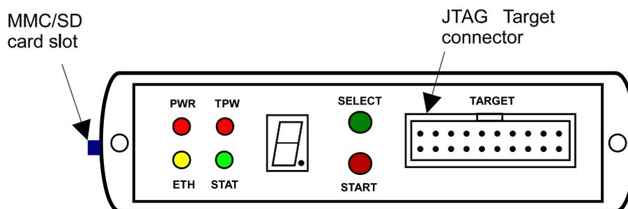
Figure 7: Rear panel connectors
