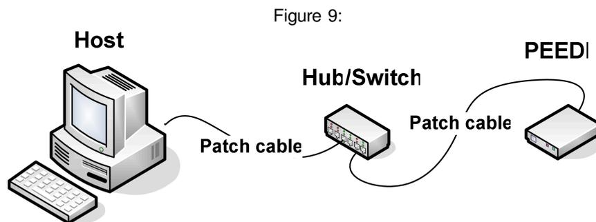
2. Connect the PEEDI interface unit to the target hardware, using the supplied JTAG adapter and cable. The JTAG adapter must be on the PEEDI side of the JTAG cable. If your target JTAG port pinout is not standard, you may need to make your own target cable considering the PEEDI JTAG connector pinout.
