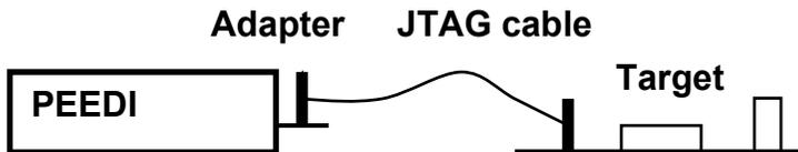
If your target JTAG port pinout is not standard, you may need to make your own target cable considering the PEEDI JTAG connector pinout.
