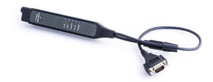
Yet more powerful and versatile a WLAN solution than Kvaser's original BlackBird, Kvaser BlackBird v2 incorporates a new radio chip that gives it up to 75% better range. In addition, more onboard memory overcomes potential interruptions to the wireless connection due to the protocol itself or disturbance.
