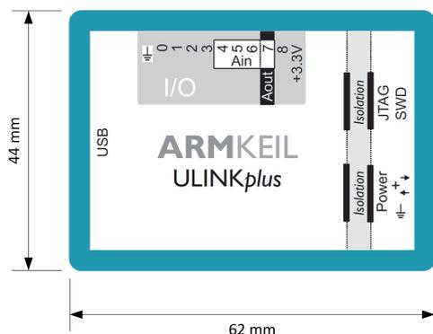
**ULINKplus** is a universal debug and trace adapter that enables test automation, software optimization for ultra-low-power applications, and isolation for debugging sensitive hardware systems. The compact enclosure allows usage in harsh environments and provides standard target connectors for JTAG, power measurement, and general purpose I/O.
