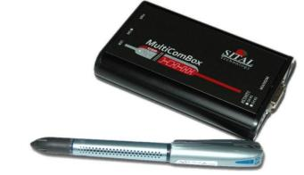
The TST1553USB unit provides full MIL-STD-1553B test, simulation and bus analysis (monitor) capability in a compact, self-contained unit. It connects via an USB 2.0 interface to any host system. The MultiComBox unit supports concurrent Bus Controller (BC) and up to 31 Remote Terminals (RT) with Bus Monitor (MT). Full error injection capability is available in BC and RT modes with full error detection in BC, RT and MT modes.
