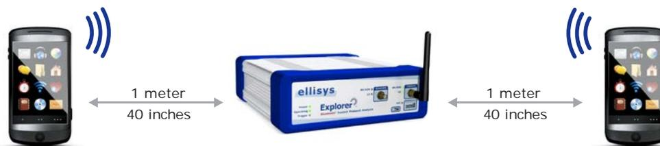
The **worst possible setup** is placing the devices very close to each other, with the analyzer far away. In this situation, the devices will reduce transmission power to the minimum, and the analyzer will receive a very small signal, which is therefore increasingly subject to interferences.
