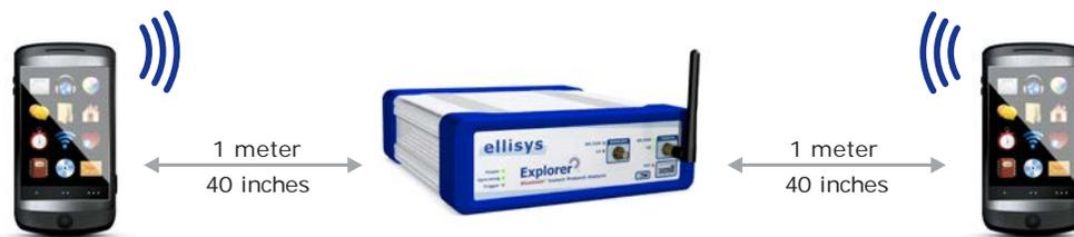
**Mobile phones lying flat:** These two mobiles phones are lying flat on a table. If the chip antenna is not specifically designed work this way, these mobile phones will have a hard time communicating.
