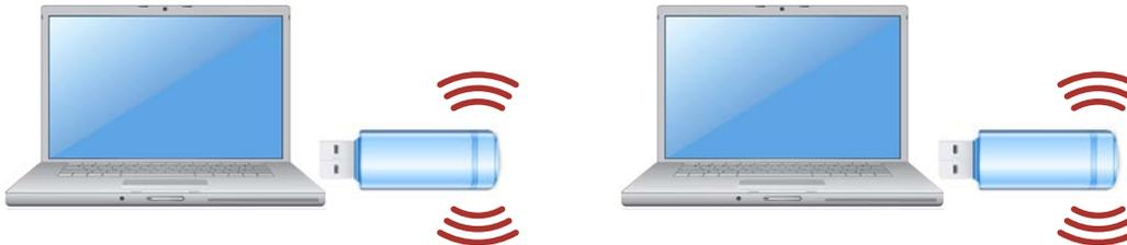
**Vertical dongle:** In this case the dongle is connected to the notebook with an adapter enabling the dongle to be operated vertically, thus positioning the antenna in its optimal position.
