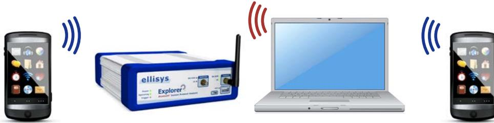
**Wireless shield:** A laptop screen is a pretty good wireless shield. In this example, it will likely interfere with the two devices, reducing the transmission quality.
