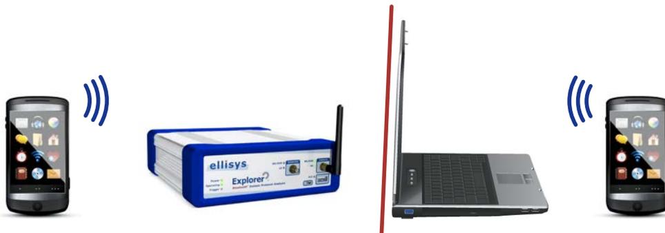
**Close devices, analyzer far away:** These two mobile phones, placed closely to each other, will reduce their transmission power to the strict minimum. The analyzer, placed far away, will receive this traffic weakly, so it will be much more sensitive to interferences, increasing the capture's error rate.
